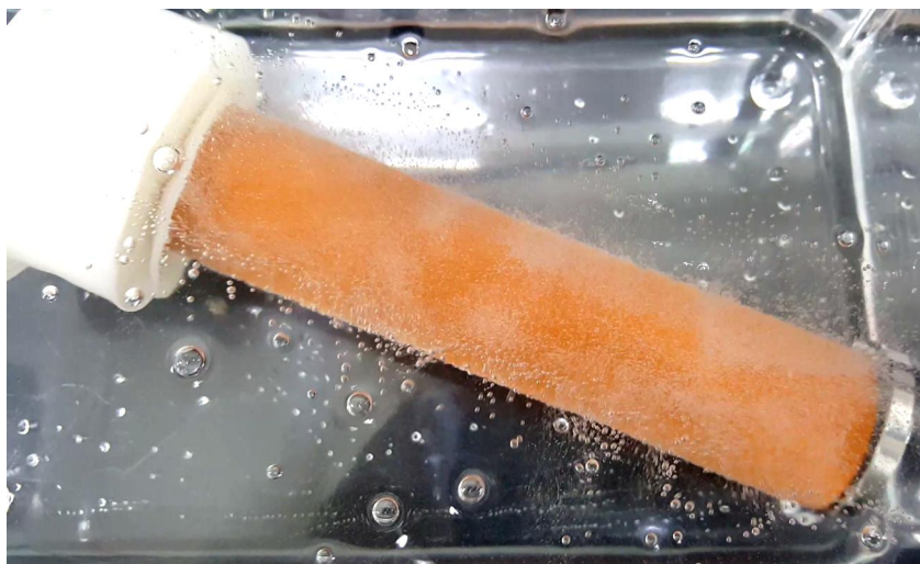
Fig. 3.2 Nucleation of Micro-nanobubbles by Ceramic Filter
